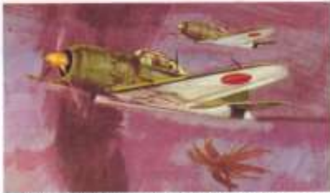
F.219F MITSUBISHI A6M ZERO-SEN This most famous of all Japanese fighters made its first flight on 1st April, 1939. Total production amounted to 10,611. It had a maximum speed of 351 mph and a range of 975 miles. It was armed with two 20 mm and one 12.7 mm cannon and 7.7 mm machine gun.
