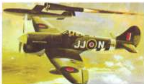
F.189F HAWKER TEMPEST MK. V The only version of the Tempest to see War service. It is best remembered for destroying 538 Flying Bombs over Southern England between June and September 1944. 805 Tempest V's were produced and they entered service in January 1944. Top speed 435 mph, range 1,530 miles.
