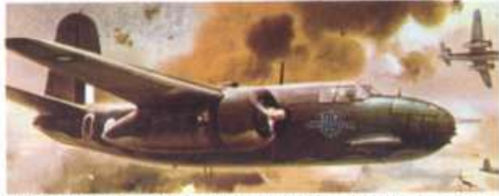
F.208 DOUGLAS HAVOC (INTRUDER) OR BOSTON This aircraft first flew in December 1938 and was the first U.S. Warplane to have a nose-wheel under-carriage. It served successfully in a wide variety of roles including attack bombing, fighting, torpedo dropping and smoke screen laying. The aircraft had a maximum speed of over 300 mph.
