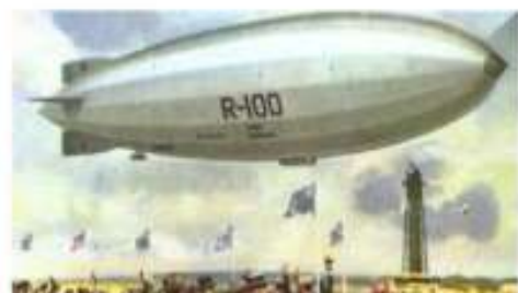
F.128 R.100 AIRSHIP (1/500th Scale) This 709 ft. long Barnes-Wallace designed Airship was launched in December 1929. In July 1930 it flew 3,242 miles from England to Montreal. It was powered by 6 Rolls Royce Condor engines.
