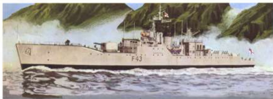
F.125 H.M.S. "TORQUAY" FRIGATE The first ship to be completed of the new "Whitby" class of Frigates designed especially for Anti-Submarine work. She was launched in 1954. She carries the very latest equipment for locating and destroying submarines including facilities for directing Anti-Submarine aircraft.
