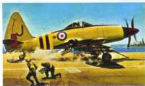
F.198 WESTLAND WYVERN The Wyvern was single-seat carrier borne strike aircraft which first flew in December 1946. Standard armament was four 20 mm cannons, a 20 inch torpedo, bombs or mines, or a combination of depth charges and rockets. It had a maximum speed of over 380 mph at sea level.
