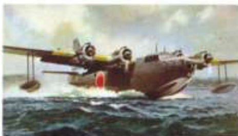
F.276 KAWANISHI H8K2 "EMILY" FLYING BOAT The largest and best Japanese Flying Boat was the superior flying boat of its day. It had a maximum speed of 282 mph and a maximum combat range of 4,474 miles. Its endurance on a single mission being anything up to twenty-four hours.
