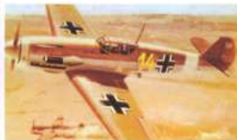
F.192F MESSERCHHMITT BF 109 First flew in 1935 and in 1937 set up a new World Air Speed Record of 379.4 mph. Many versions were produced and they became the main service fighter of the Luftwaffe during the War. The 109G had a top speed of 428 mph and a range of 350 miles.
