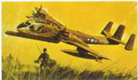
F.270 GRUMMAN OV-1B MOHAWK This aircraft first flew in 1959 and is still operational to-day. Planned solely as a reconnaissance aircraft it has two turbo-prop engines and can travel at low speeds for considerable periods of time. It is equipped with side looking airborne radar.
