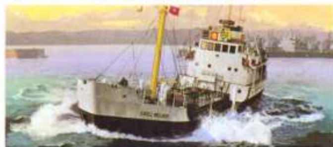
F.137 SHELL COASTAL TANKER Our model is typical of the many small coastal tankers which operate all over the world. This ship, built in 1955, is 586 tons deadweight with a displacement of 1,042 tons and is 117 ft. 11 in. long. She is sailed by her Master and a crew of ten.
