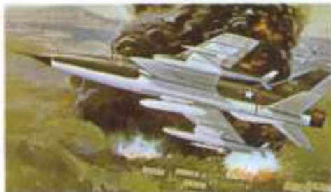
F.269 REPUBLIC F-105 THUNDERCHIEF This excellent fighter-bomber first flew in October 1955 and was to become the heaviest single-seater to enter service with the U.S.A.F. It had a maximum speed of 1254 mph with a combat range of 1840 miles and was capable of carrying a bomb load of 12,000 lb.
