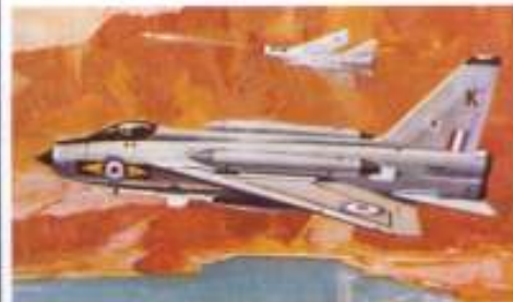
F.266 B.A.C. LIGHTNING F.5 This single-seat twin-engined all weather fighter can exceed the speed of sound in level flight and it was the first fully supersonic aircraft in service with the R.A.F. Armed with cannon, rockets, bombs or missiles and travelling like "Lightning", it is the last word in defence aircraft.
