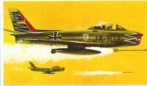
F.267 NORTH AMERICAN SABRE Destined to become one of the truly great combat aircraft of all time, this aircraft, the first swept wing fighter of the USAAF first flew in October 1947. It had a top speed of 680 mph and a range of 920 miles.
