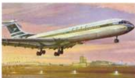
F.140 B.A.C. SUPER VC.10 This aircraft is powered by four Rolls Royce Conway RCO 43 Turbo-fan engines and has a maximum cruising speed of 581 mph. Over fifty VC. 10's have been produced and they have flown over 300,000,000 miles in five years.
