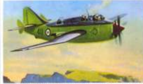
F.331 FAIREY GANNET Developed as an anti-submarine search and strike aircraft, the Gannet was powered by the unique Armstrong-Siddeley Double Mamba power plant which could run on Kerosene or Diesel fuel and which helped the Admiralty to eliminate petrol from carriers. It had a top speed of 300 mph.
