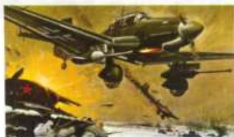
F.195 JUNKERS JU87 STUKA This famous dive bomber could release its bombs from a near vertical dive. Although not technically a good plane, it was remarkably successful in the early stages of the War and this model was particularly developed as an anti-tank version with two 37 mm underwing cannons.
