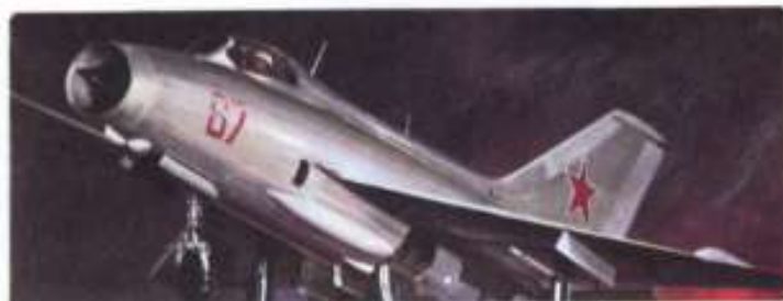
F.263 MIG 21 "FISHBED" This short-range clear-weather fighter, appeared in 1956 at the Soviet Aviation Day display in Moscow. It has a maximum speed of 1320 mph and a combat range radius of 375 miles. It serves in the Air Forces of at least 14 countries.
